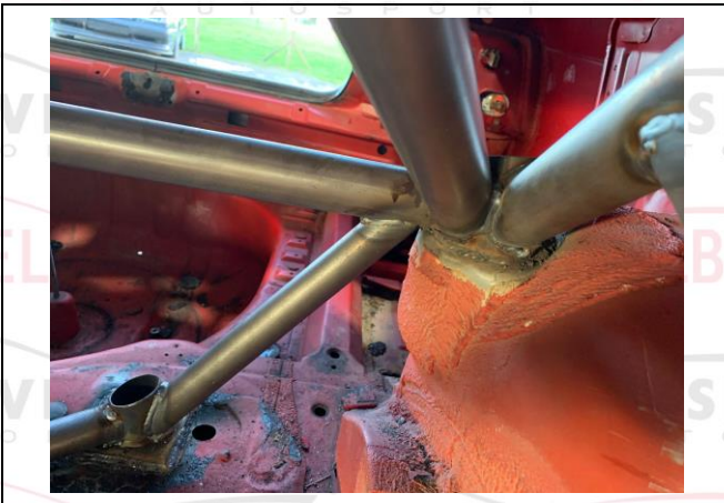
PHOTO 5 REAR BACKSTAY TO BODYSHELL ATTACHMENT
