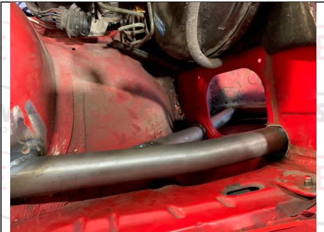
PHOTO 9 ATTACHMENT TO FRONT SUSPENSION
