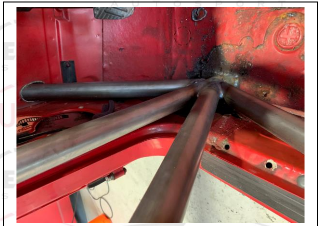
PHOTO 6 FRONT ROLLBAR TO FLOOR ATTACHMENT
